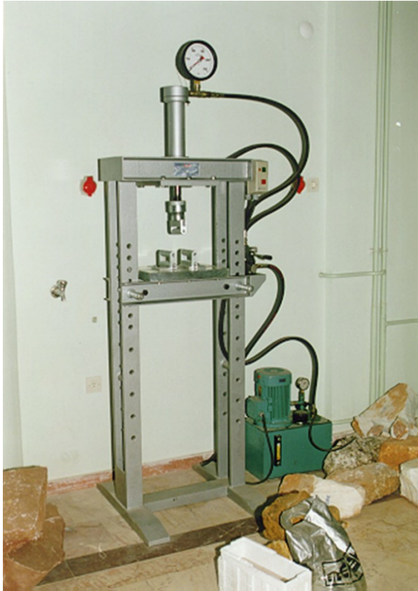
1.Marble and Rock Mechanics Laboratory- Flexural Strength Tester /2. Losangelas Measuring Tool
