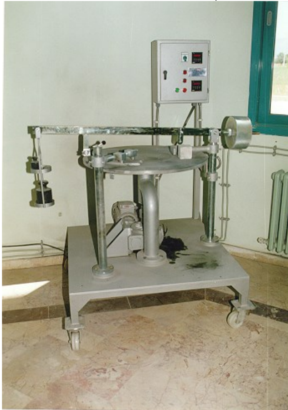
1.Marble and Rock Mechanics Laboratory-Böhme Surface Wear Gauge/2.Point Loading-Oven
