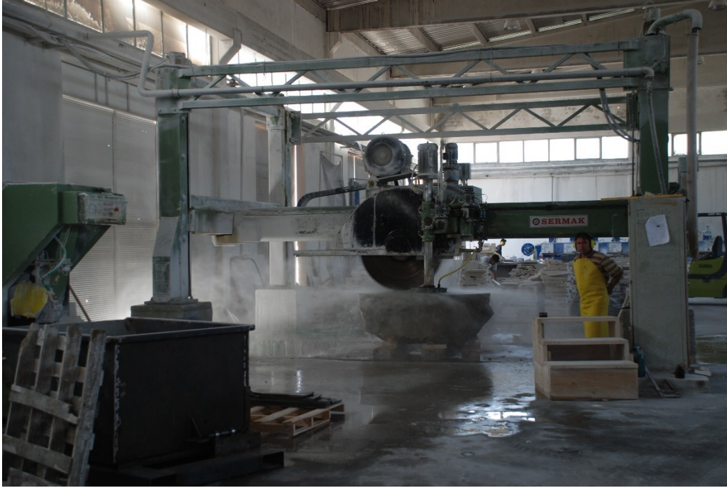
Marble Factory 30cmXLength free -Strip Cutting / 4 Legs S/T Machine Application
